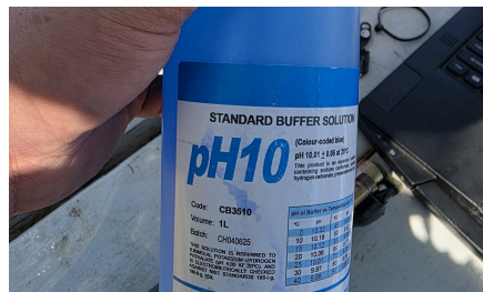
pH calibration with certified buffer
