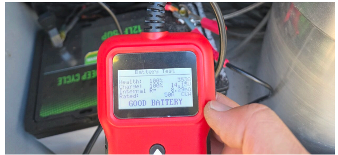
Battery load test
