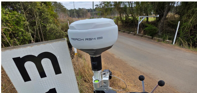
Gauge board surveyed to AHD with RTK GNSS
